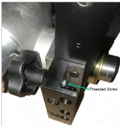
Rail Drill Rail Shoe Location
