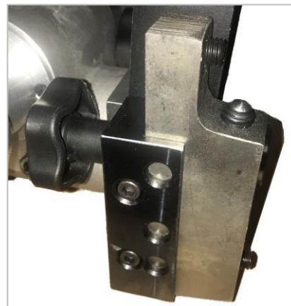
Properly Installed Rail Shoe
